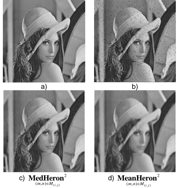
Fig. 1. Original (a) and noise (b) images. Denoised images (c) and (d).
